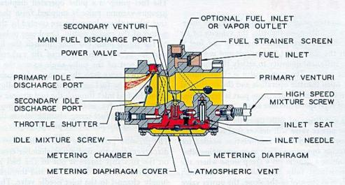
The model HD carburetor is also available with a plain diaphragm cover plate. The fuel must come from a separate fuel pump or an overhead fuel tank for a gravity fuel supply for these two optional models.
