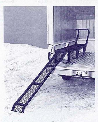
This unit is designed to fit all long-wide-box pickups. Measure the width of pickup to make certain you have ample room before starting construction. We show basic ramp and carrier. Photo at left shows additional items such as front stop and hold-down chains you may wish to add.
